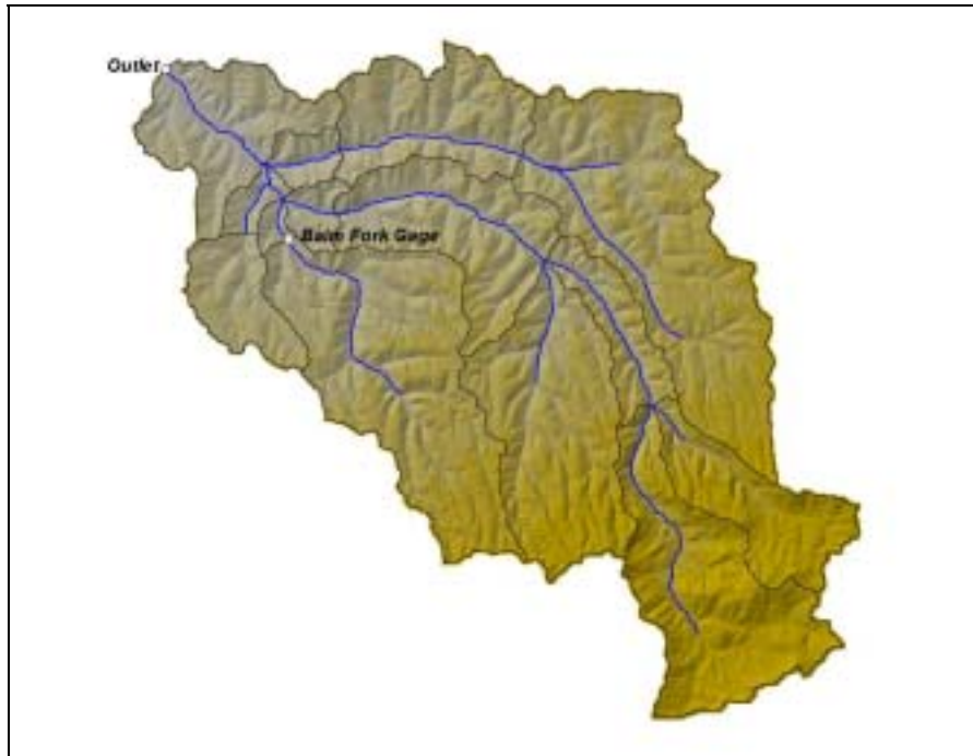
Figure 4: Topographic map and basin model of the Heppner, Oregon, watershed created by HEC-GeoHMS.
